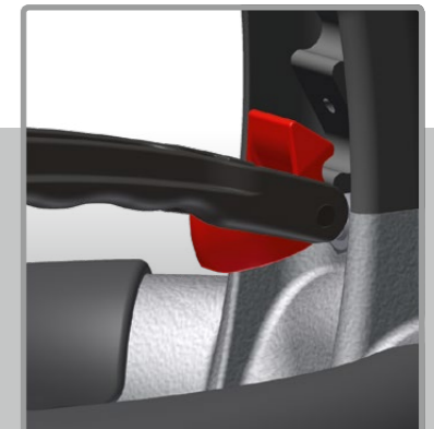
LeverAssist® reduces hold-open force by 75 %.
