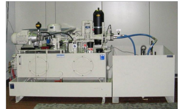
Pressure Impulse Test Rig
